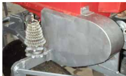
Fig 3. Similar hazard securely guarded Note: Gear wheels visible are inoperative
